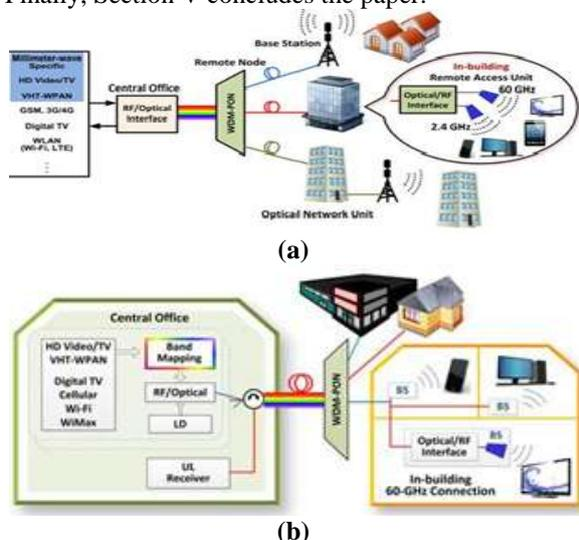
Fig. 1. System architectures of (a) all-band RoF and (b) band-mapped 60-GHz RoF for the unified multi-service optical-wireless access networks.
