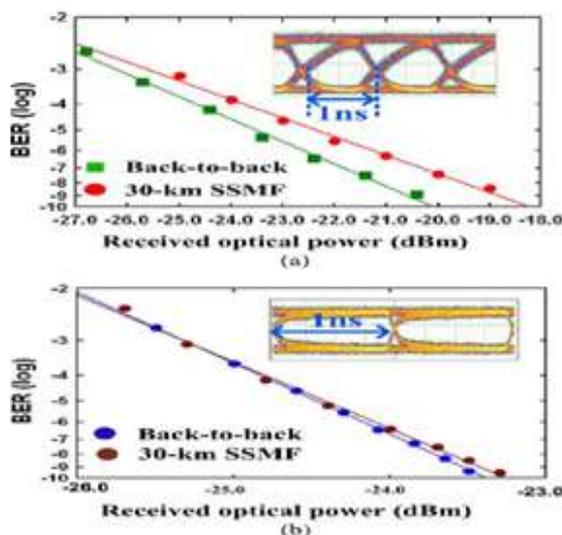
Fig. 4. BER performances and eye diagrams for the (a) downconverted mm-wave signal and (b) the upstream signal
